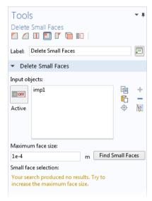
5 Use the Zoom to Selected button next to the list to find the faces on the rim, which are found around the bolt holes, as illustrated in the figure below.
