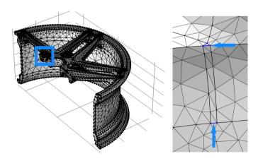
The short edges in this region form a small face which you remove using the *Collapse Edges* operation. The long edges of the sliver face can be removed by adding them to the existing Ignore Edges 1 operation in the geometry sequence.
