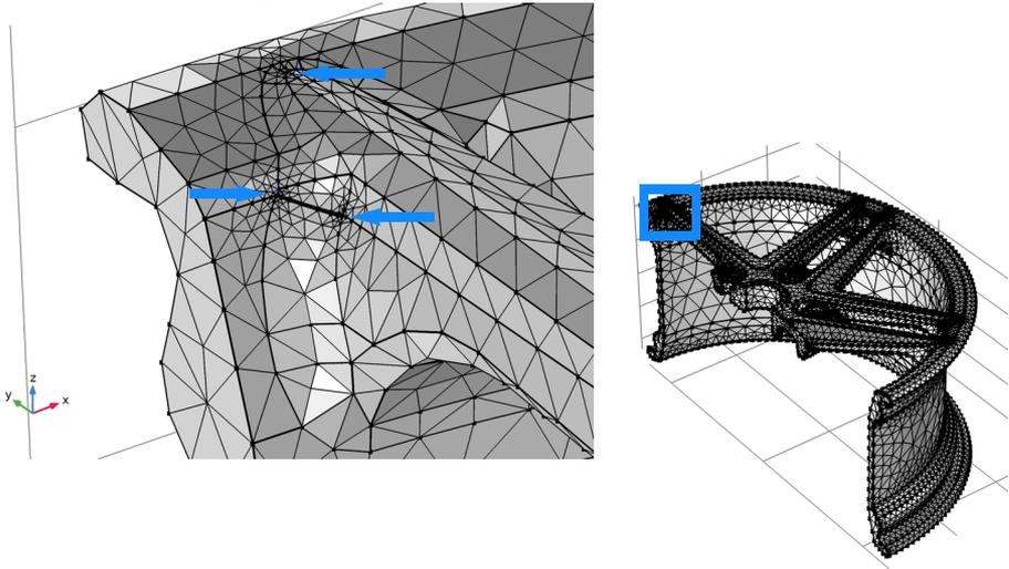
On closer examination you can see that several edges in this area are highlighted as being too short to be meshed with the current mesh settings.
