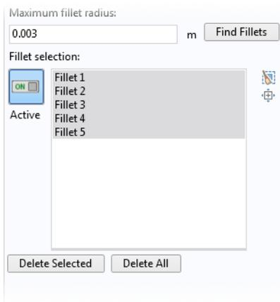
As the operation completes and the fillets are removed note that the Delete Fillets 1 (dfi1) node is inserted into the geometry sequence, just above the Cap Faces 1 (cap1) node. The Cap Faces 1 (cap1) node is still unavailable, meaning that it is currently not built.
