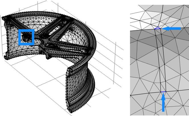
The short edges in this region form a small face which you remove using the *Collapse Edges* operation. The long edges of the sliver face can be removed by adding them to the existing Ignore Edges 1 operation in the geometry sequence.
