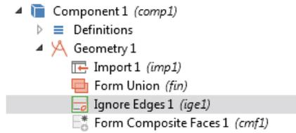
A green rectangle is displayed around the Ignore Edges 1 node telling you that this is the current node. Any operations that you add to the sequence are placed directly after the current node. The Form Composite Faces 1 (cmf1) node is marked, which indicates that the node needs rebuilding.
