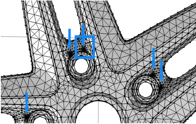
The areas of dense mesh, indicated by the arrows in the figure, are due to slivers and small faces. Zooming in even closer inside the blue rectangle reveals a small triangular face sitting adjacent to a sliver face. Two of these can be found around each bolt hole location. The edges that are highlighted in blue are listed in the Selection list of the Warning window.
