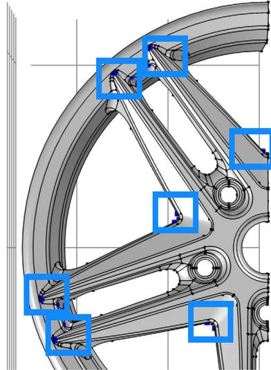
The resulting geometry is similar to the one after the last repair operation in the previous tutorial. The difference is that using the defeaturing tools you can have more control over which entities to delete and in which order.
